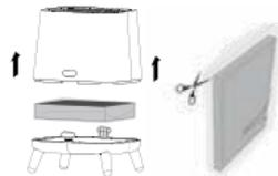
3. Put the filters back, making sure the arrows are in the right direction
